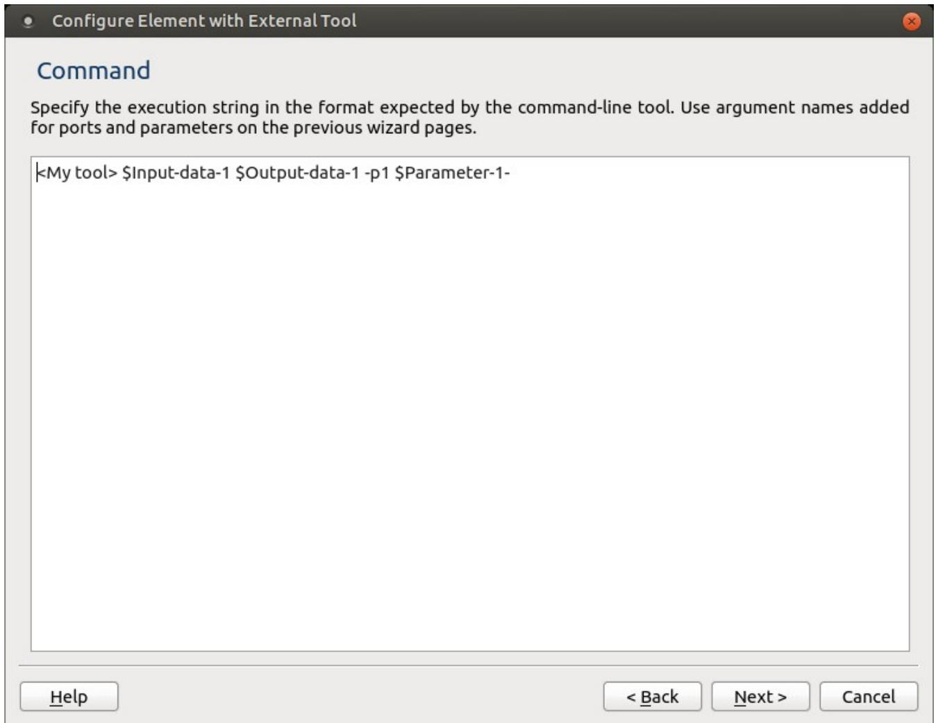
The signature of the execution string depends on the command that is launched. But the general rule is that input/output data and attributes have prefix \$. You can set the parameterized description for the new element (the description that appears not in property editor but on the element itself). In the parameterized description, you also can use parameters substitution with prefix \$. If the paths in the execution string contain spaces, they must be enclosed with quotes.
